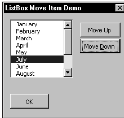
Figure 14-13: The buttons allow the user to move items up or down in the ListBox.
