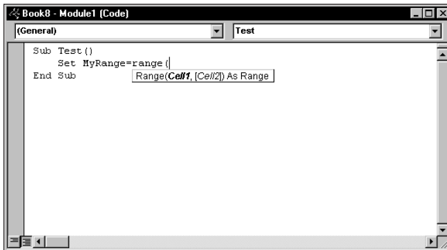
Figure 7-10: An example of Auto Quick Info offering help about the Range property.
