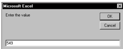
Figure 11-3: The InputBox function gets a value from the user to be inserted into a cell.
