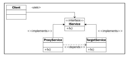
A proxy is usually implemented by using a common, shared interface or super class. Both the proxy and the target share this common interface. Then, the proxy delegates the calls to the target class.
