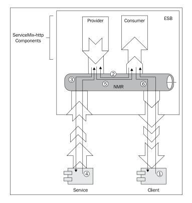
The above figure shows two instances of servicemix-http deployed in the ServiceMix ESB, one in a provider role and the other in the consumer role. As it is evident, these roles are with respect to the NMR of the ESB. In other words, a
