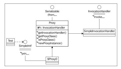
The above figure shows the relationship between various classes and interfaces in the sample. \$Proxy0 class represents the actual proxy class generated on the fly and as you can deduce it from the class diagram. \$Proxy0 is a type of our interface (SimpleIntf). To build the sample, first change directory to ch13\JdkProxy and execute ant as shown here:
