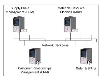
The following figure represents systems that are autonomous, but federated to facilitate information flow:
