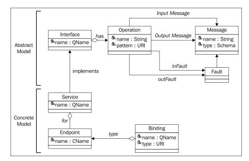
The following figure represents the two parts of the WSDL representation of a service:
