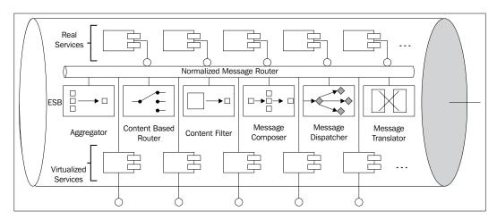
This figure depicts the concept of Service Virtualization, where we make use of core ESB features like Aggregation, Routing, and Translation to republish the existing service assets. These are explained in detail in subsequent chapters.
