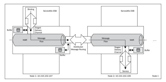
• JCA Flow: The ServiceMix JCA NMR flow is very much similar to the JMS flow. In fact, ServiceMix uses JMS sessions as the underlying mechanism so that multiple ServiceMix containers can collaborate in a cluster. In addition, JCA provides support for XA transactions when sending and receiving JBI exchanges.
