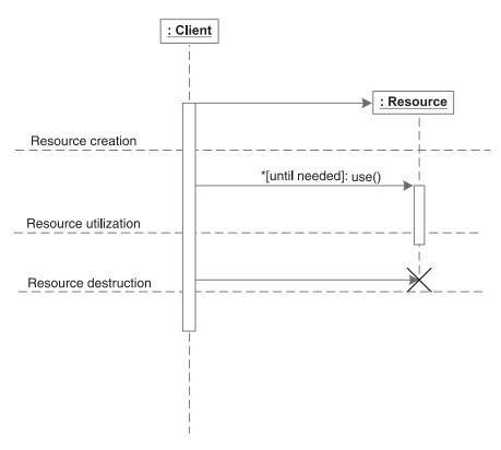
Figure 7.1 Typical resource usage in the absence of any pooling. You create resources just in time to serve the requests, use them, and dispose of them after their usage. Any subsequent use requires creating a new resource.
