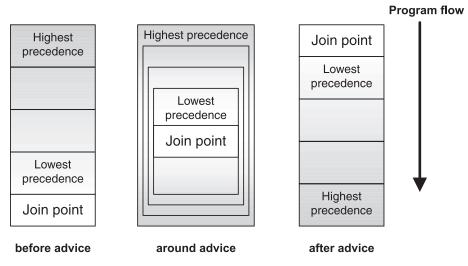
Figure 4.2 Ordering the execution of advice and join points. The darker areas represent the higher-precedence advice. The around advice could be thought of as the higher-precedence advice running the lower-precedence advice in a nested manner.
