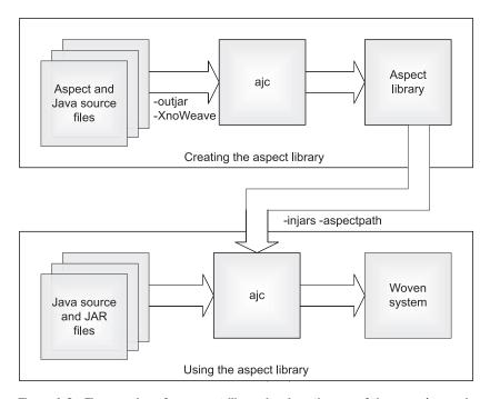
Figure A.2 The creation of an aspect library involves the use of the -outjar and -XnoWeave options. When you use the library, you need the -aspectpath and -injars options. The output of the system could be multiple class files or a JAR file, depending on how you use the -outjar option.
