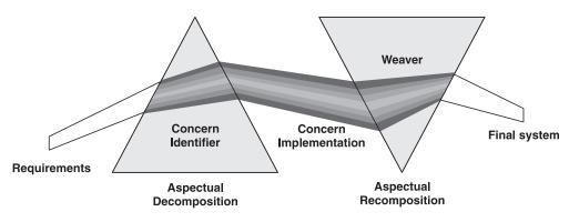
Figure 1.10 AOP development stages. In the first stage, you decompose the system requirements into individual concerns and implement them independently. The weaver takes these implementations and combines them together to form the final system.
