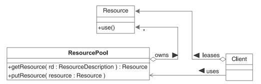
Figure 7.2 The structure of a resource pool, resource, and client. The resource pool owns the resources in it, and the client leases a resource from it.
